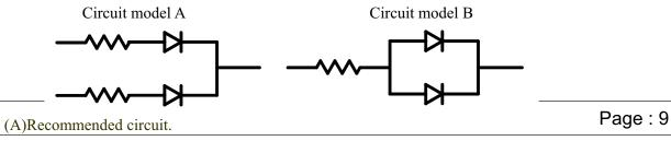
(B)The difference of brightness between LED's could be found due to the Vf-If characteristics of LED.
